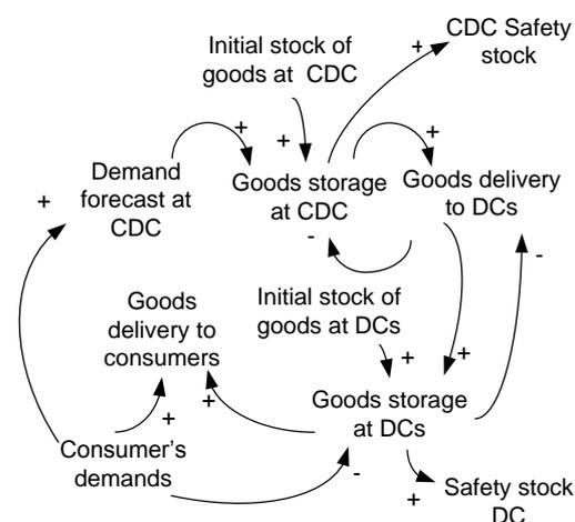
Figure 2. The causal loop diagram of distribution sub-models
