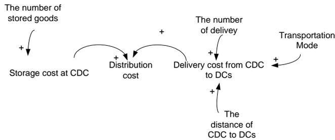
Figure 3. The causal loop diagram of distribution cost sub-model
