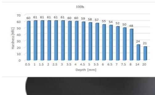
**Fig.7** Diagram of hardness for SAE3310 after 100 hours
